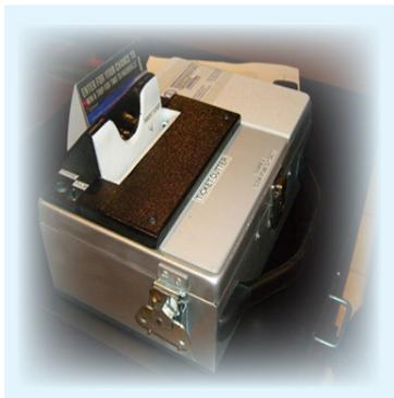
Kevin was not able to tear movie tickets, and he needed some way to do this job duty. Initially he tested a “ticket cutter box” made by a rehabilitation engineer at the Virginia Department for Aging and Rehabilitative Services (VA DARS). The box had a blade attached to a sensor that cuts the tickets in half when inserted. Due to a number of design concerns and Kevin’s individual needs, the rehabilitation engineer made modifications. The resulting ticket cutter is shown in the photo.
