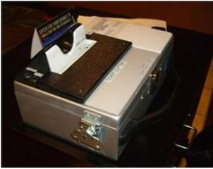
Kevin was not able to tear movie tickets, and he needed some way to do this job duty. Initially he tested a “ticket cutter box” made by a rehabilitation engineer at the Virginia Department for Aging and Rehabilitative Services (VA DARS). The box had a blade attached to a sensor that cuts the tickets in half when inserted. Due to a number of design concerns and Kevin’s individual needs, the rehabilitation engineer made modifications. The resulting ticket cutter is shown in the photo.
